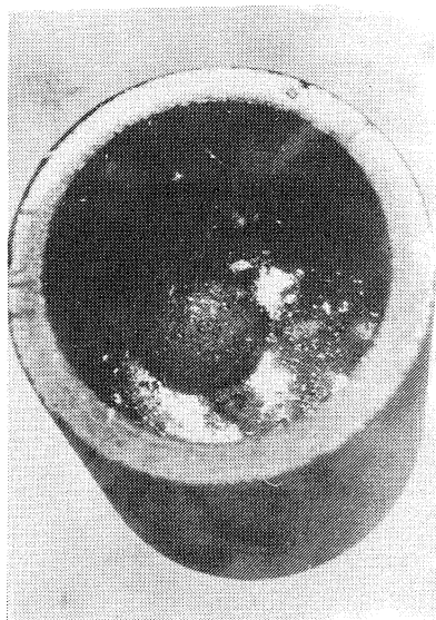
Fig. 7. An appearance of the graphite crucible just after the growth of graphite single-crystal film for Run No. (S-1-17).
